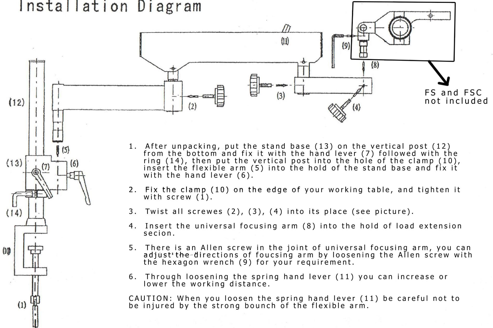
1. After unpacking, put the stand base (13) on the vertical post (12) from the bottom and fix it with the hand lever (7) followed with the ring (14), then put the vertical post into the hole of the clamp (10), insert the flexible arm (5) into the hold of the stand base and fix it with the hand lever (6).
